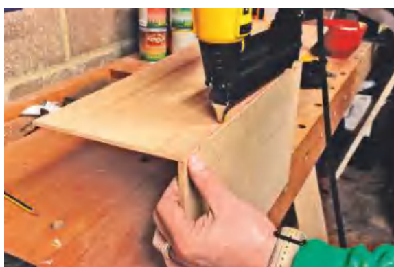
The Precision Point makes it very easy to align on thinner stock
